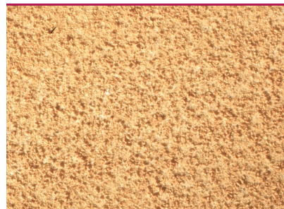
Alm. Borebille - boremel. (Foto: Protox)
